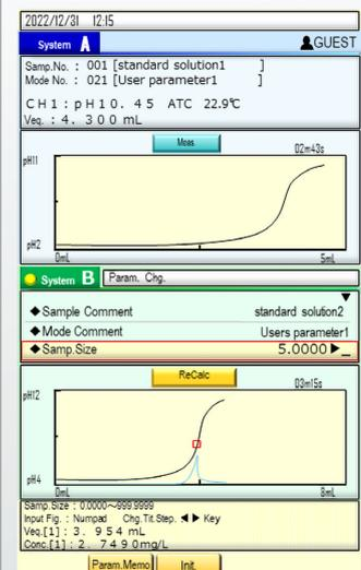
Simultaneous display and titration of system A and B are supported. Viewing data and reanalyzing is available from one system while measuring with another.
