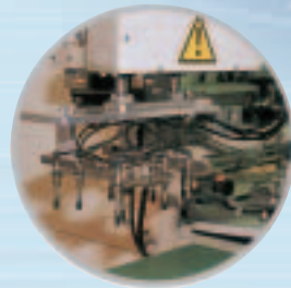
Pick & Place for Loading/Unloading PC Board.
