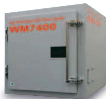
A shield box and a chamber box are required for accurate EMC testing. The photo shows a shield box (sold separately) designed exclusively for our WM7400.
