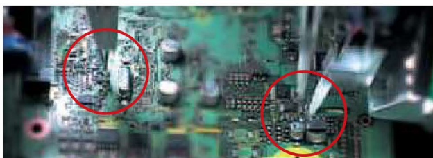
Worry-free probe contact even in locations that are densely populated with components
