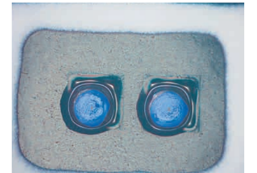
0402 laminated ceramic pad at 200x
