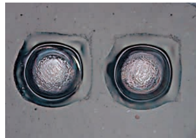
0402 laminated ceramic pad at 200x
