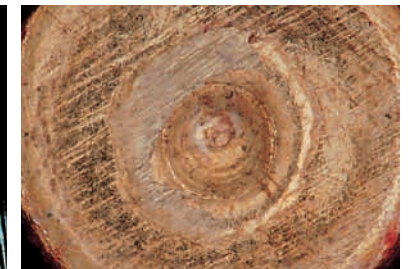
Bullet, impression after use, at 50x
